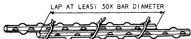
Figure 7-31.-Bars spliced by lapping.
